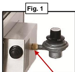
Screw the brass nut of the regulator into the side of the control box.
